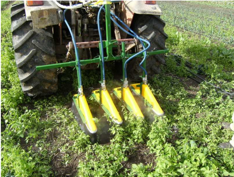
Figure 3. Tractor-mounted applicator for steam weeding.
